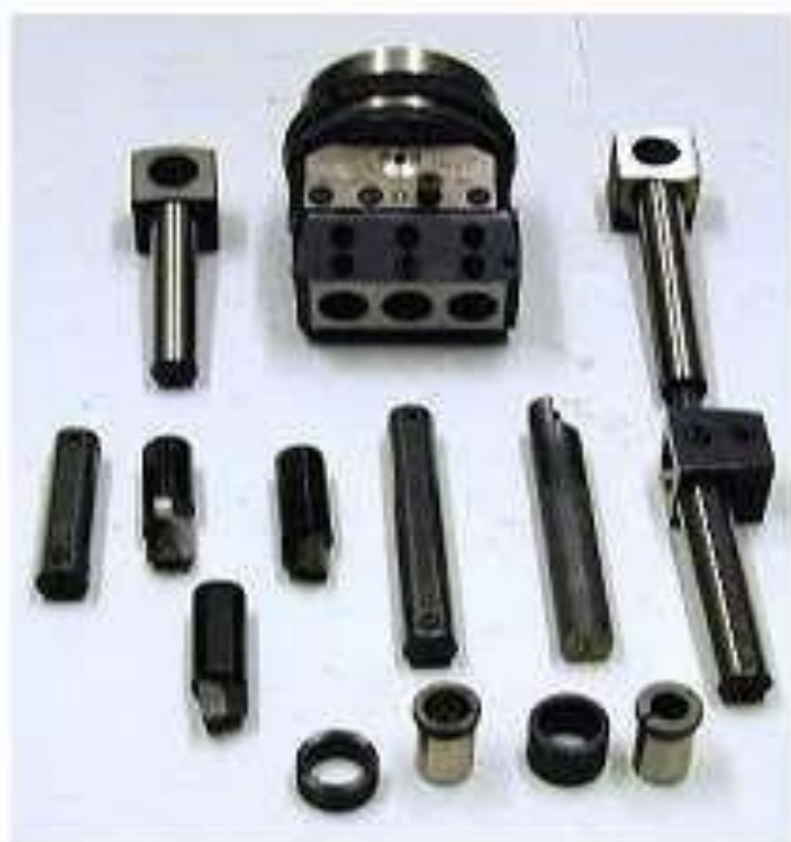
Boring bar with indexable carbide insert ( Left ), and adjustable boring head with accessories ( Right ).
